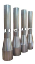
Standard Transvac Tank Jet Mixers entrain 3 parts suction liquid for every 1 part motive liquid with the discharge jet of 4 parts inducing further secondary mixing.
