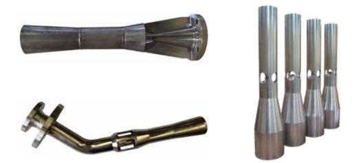
Standard Transvac Tank Jet Mixers entrain 3 parts suction liquid for every 1 part motive liquid with the discharge jet of 4 parts inducing further secondary mixing.
