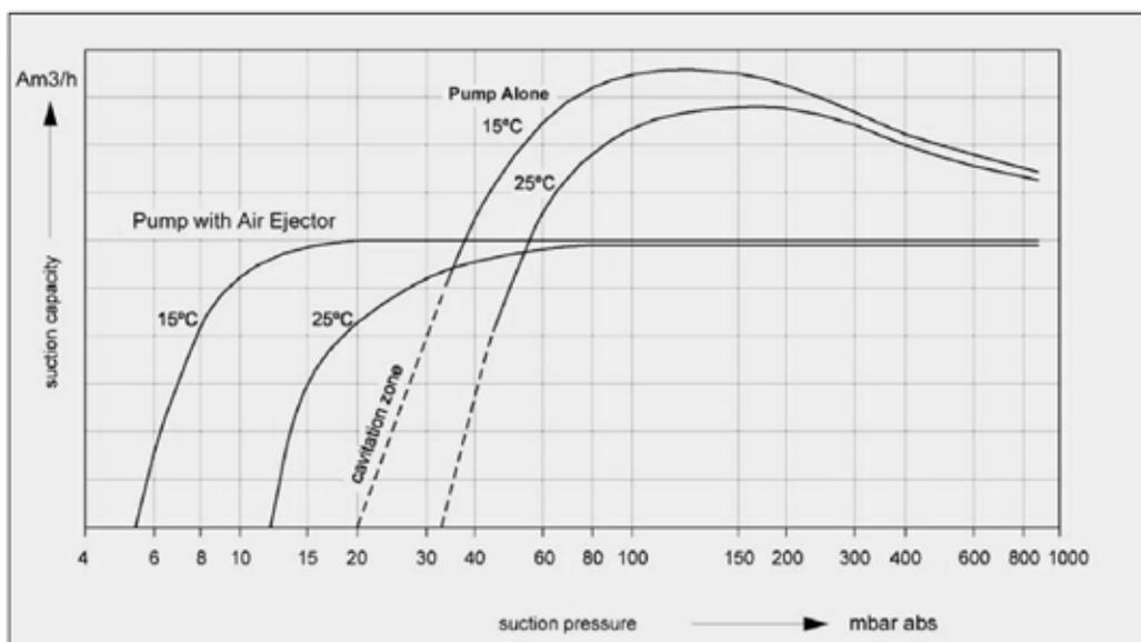
The chart above shows the typical performance of a 2 stage Liquid Ring Pump operating alone with seal water at temperatures of 150C and 250C and when operating in combination with an Atmospheric Air Jet Ejector. A by-pass line can be installed around the Ejector when evacuation times are critical. All Transvac Ejectors are custom designed to suit each application to ensure maximum operating efficiency.
