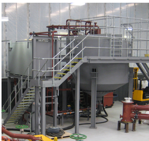
Sellafield sand slurry rig, purpose built for nuclear Ejector testing
