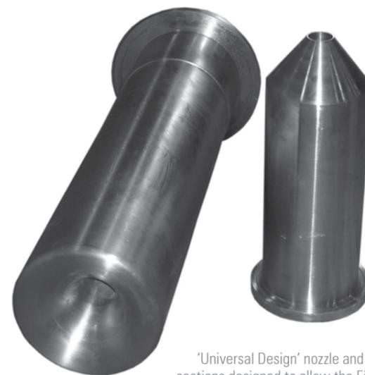
'Universal Design' nozzle and diffuser sections designed to allow the Ejector to operate at new production conditions
