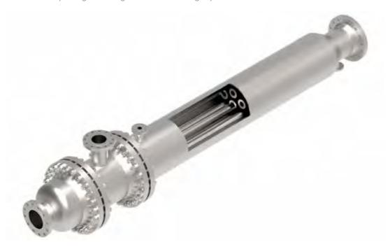
There is one common inlet on the high pressure motive side, which feeds into multiple nozzles. In turn these nozzles then discharge into a common suction chamber where the low pressure suction stream is introduced. Finally, this combined flow is sent through a number of diffusers to a common, single LJC outlet connection.
