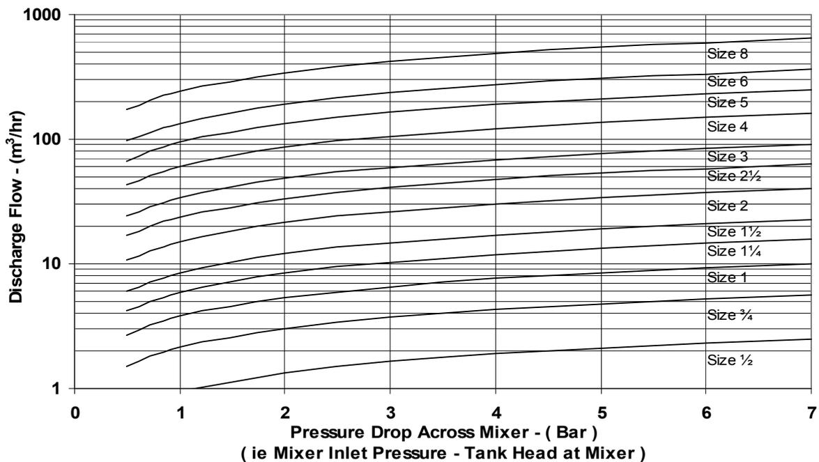
A Transvac Tank Jet Mixer can normally be employed on any application in which the process liquid is capable of being handled by a centrifugal pump. Factors considered in selection include tank volume, viscosity, specific gravity, size and percentage of solids as well as tank geometry.
