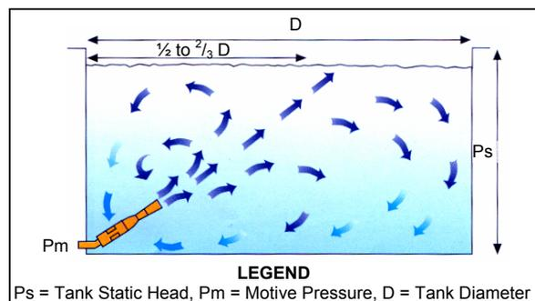
As the resulting mixture passes through the diverging cone its velocity is partially reduced to regain sufficient pressure to overcome the static head of liquid within the process tank. At the discharge a high energy, turbulent jet is emitted entraining and absorbing surrounding liquid at its boundary, thus creating additional currents and turbulence to ensure complete mixing of the process tank contents.
